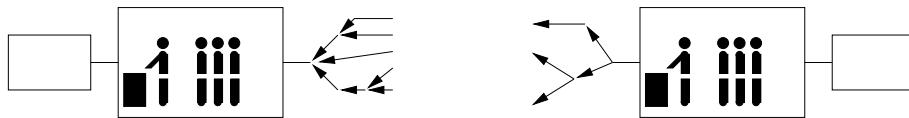
Figure 3.6: #adapt_multi bricks pose an extreme bottleneck wherever they are placed. At the left border of the brick network (near original resource providers), there is a potentially high load of incoming operation invocations that can only pass one-by-one. At the right border (near “application” bricks), an operation may take a relatively long time and make other operations wait for it.
